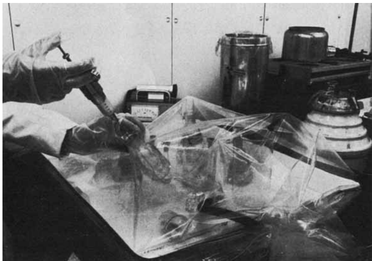
Fig. 1 Technique for handling small quantities of aluminium alkyls in an inert atmosphere.
